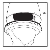
d. Push the lower dome inside the back box, line up the mounting screw holes, and install the two mounting screws.
